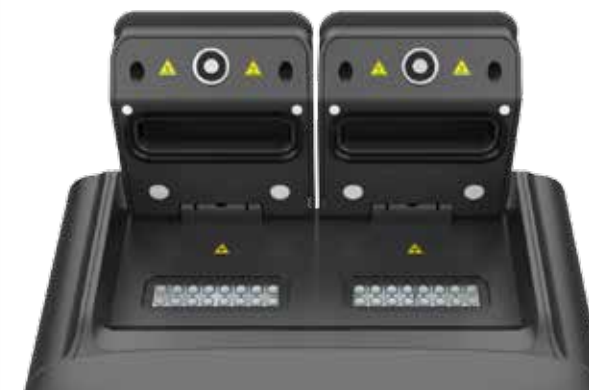
4 Channels & Double 16-Well Blocks Design, can run two different programs at the same time
